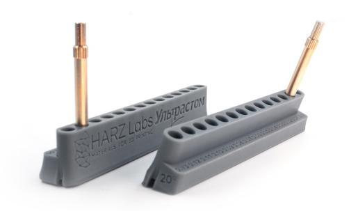
This way you can select the optimal gap for your printer and material and use it when modeling your work. Please note that a significant deviation of the mounting hole from the Z axis can lead to ovalization of the hole and the impossibility of installing an analogue. In such cases, it is worth returning to setting up the printer using a calibration test and adjusting the operating modes. In some cases, you can use compensation along the Z axis, which levels out the ovalization of the hole.
