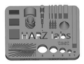
Using it, you can individually adjust the operating modes of the material and evaluate the detailing. Print results depend not only on the parameters and settings, but also on the capabilities of the printer. Not all printers are able to qualitatively polymerize material while maintaining acceptable detail. Good polymerization, in turn, avoids shrinkage and deformation over time.
